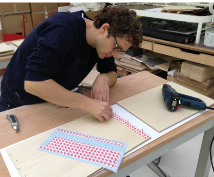
Dominik Hammer exploring a possible technical solution to glue polypropylene hinges onto veneer wood using a specific double-sided tape
