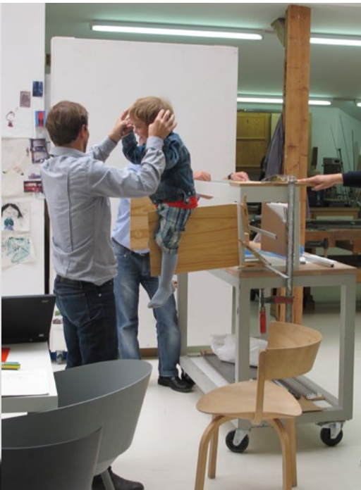
Quick stability test of the living hinge, which is holding the sliding door
