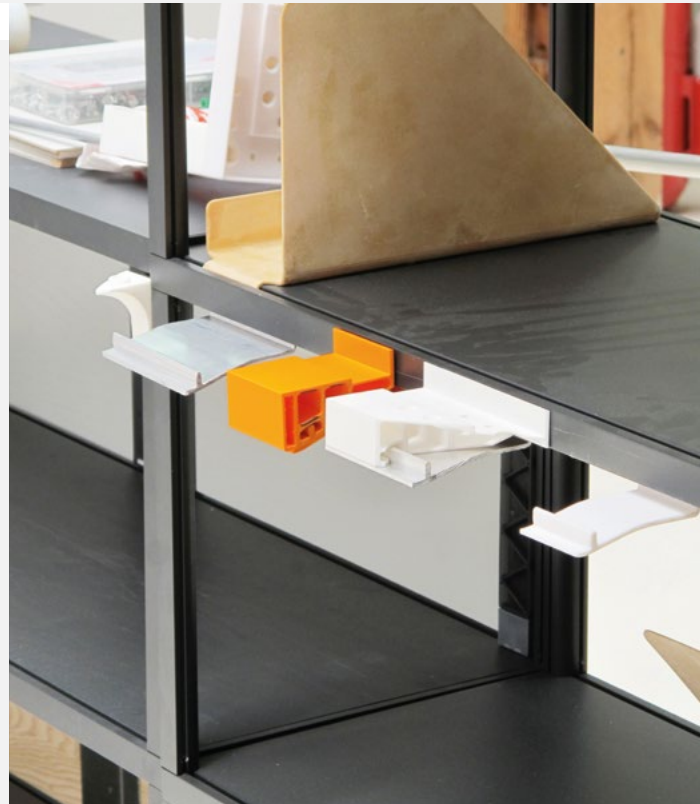
SLS models for testing the connection between table profiles and shelves
